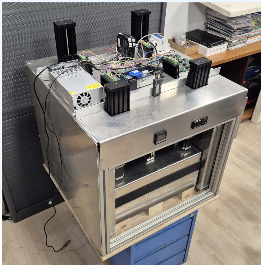
Testing device to verify thermal conductivity. Picture provided by La Rue ASBL
